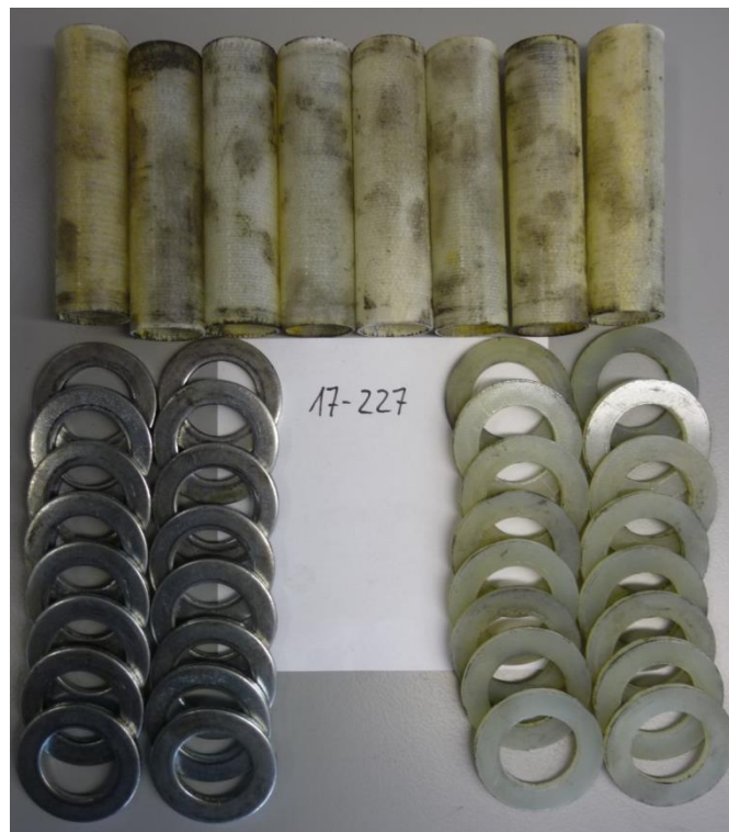
Shell electrical isolation test according MESC SPE 85/300 - 3.3.15 Insulation Gasket K/# KINS-HA (insulation gasket kit)
